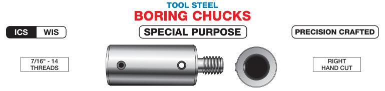
Boring Chucks are designed for use in machines requiring a 7/16"-14 threaded shank. They accept straight shank drills and are held in place with set screw(s). Each chuck has a 3/16" or 1/4" hole through the body to tighten the threaded shank into the drilling machine holder. They are also known as Adapter Chucks and are compatible with Morris Adapter Chucks (style 1) and Forrest City Boring Chucks (#5).
