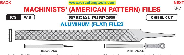
Aluminum Flat Files are designed with a special tooth construction for filing aluminum and other soft metals with a minimum of clogging. They are double cut and tapered in width and thickness.
